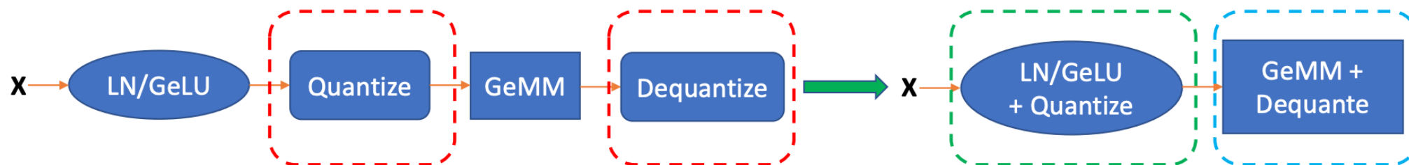
Figure 2: The illustration of normal (left) and our fused (right) INT8 GeMM.
