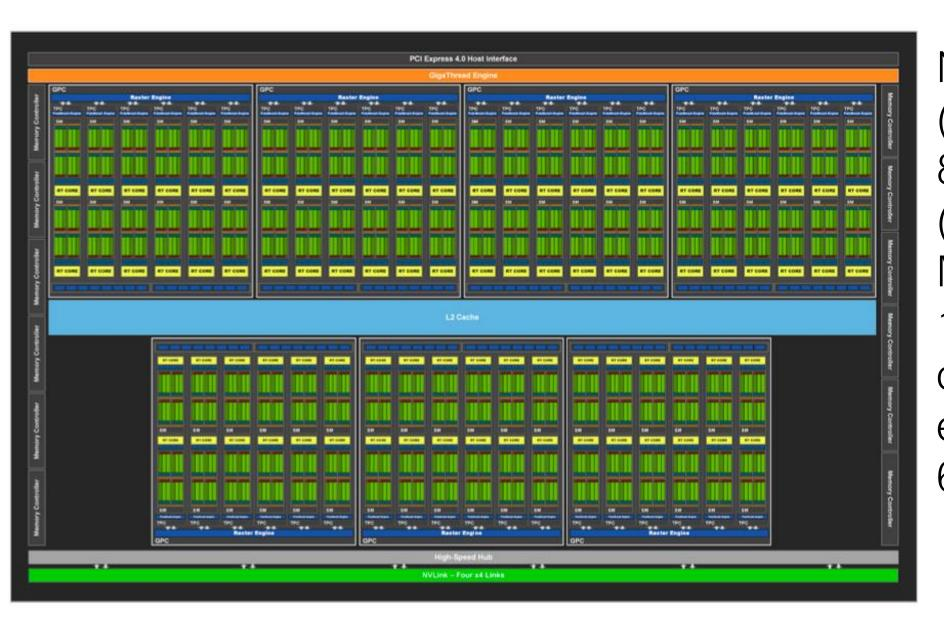
Nvidia RTX A6000 (GA102) 84 SMs (Streaming Multiprocessors) 12 memory controller (32bit ea.) total 384bit. 6MB L2 cache.
